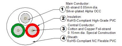
All conductors are nonmagnetic, rhodium-plated and treated with Furutech's  $\alpha$  (Alpha) process
